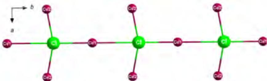
Figure 2. Cl– $\text{Ce}^{3+}$  partial structure of  $\text{Ce}_3\text{Cl}[\text{SiO}_4]_2$  with infinite chains  $1\text{D}-\{[\text{ClCe}_{2/1}^{\text{t}}\text{Ce}_{2/2}^{\text{v}}]^{8+}\}$ .
